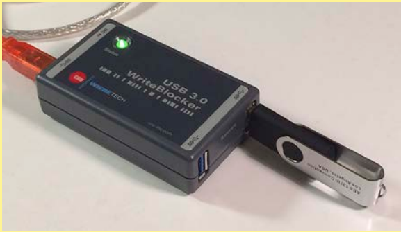
Fig. 3. A “write blocker” can be used to prevent anything being altered on a USB stick being examined. (Courtesy Eddy Brixen)
